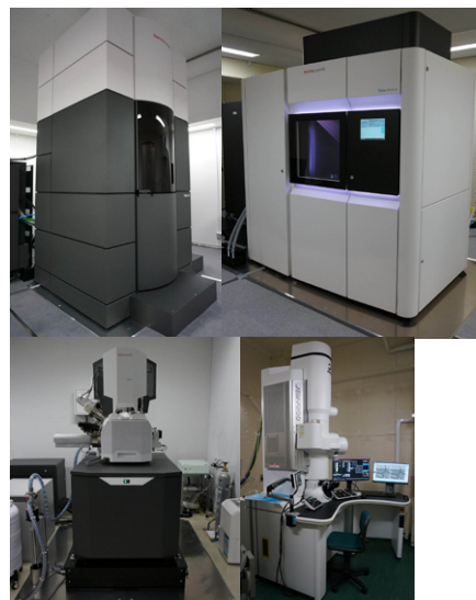
Cryo-electron microscopies installed in the University of Tokyo. From left to right: Titan Krios G3i (upper left), Talos Arctica (upper right), Aquilos (FIB-SEM, lower left), JEOL JEM-F200 (lower right).
