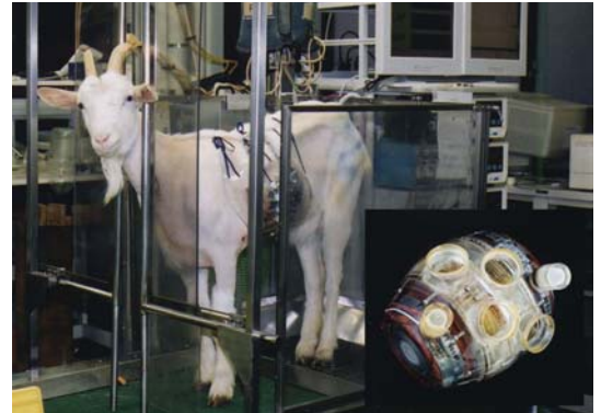
Implantable total artificial heart (Undulation pump total artificial heart) and artificial heart animal (goat)
